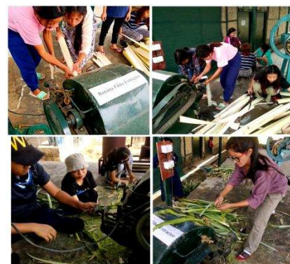
Extraction of fibre using the fibre extractor machine
